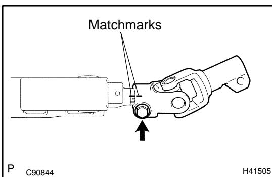
**22. REMOVE STEERING SLIDING YOKE SUB-ASSY**
