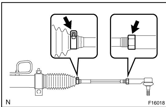
(3) Remove the RH and LH boot clips from the rack boots.
