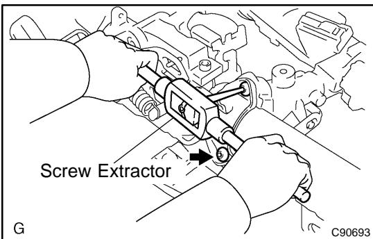
**24. REMOVE STEERING COLUMN UPPER W/SWITCH BRACKET ASSY**
