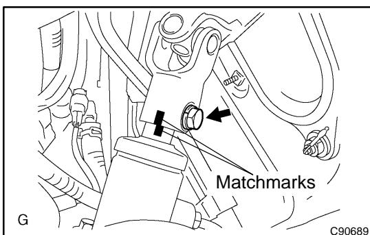
**21. REMOVE STEERING INTERMEDIATE SHAFT SUB-ASSY**
