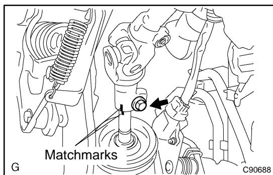
**18. DISCONNECT STEERING SLIDING YOKE SUB-ASSY**
