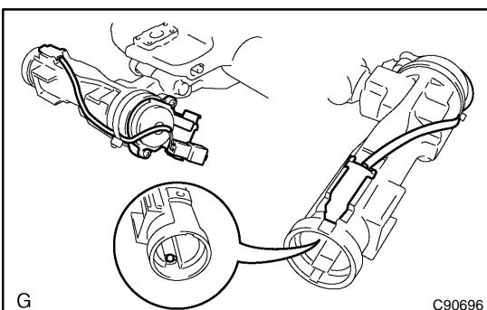
**26. REMOVE UN-LOCK WARNING SWITCH ASSY**
