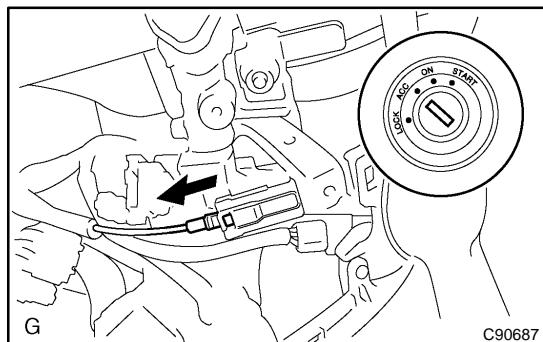
**17. DISCONNECT FLOOR SHIFT PARKING LOCK CABLE ASSY**
